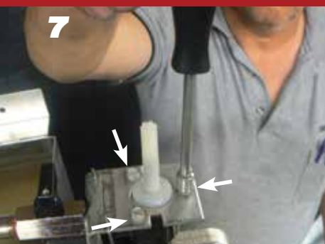
7 With 1/4" Nut Driver remove the 3 screws that hold Valve Body to Bracket.
