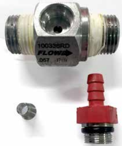
Crud and soap buildup can prevent chemical draw
