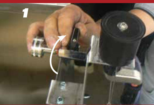
1 Turn water valve off at Hydrominder Inlet.
