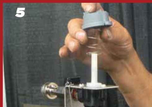
5 Remove Magnet and Magnet Spring.
