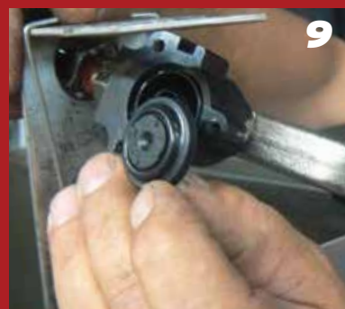
9 Remove Diaphragm from Valve Body. Inspect, clean or replace Diaphragm.
