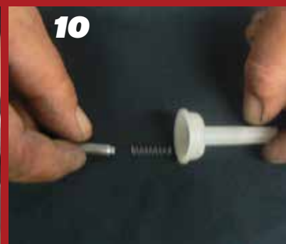
10 Inspect, clean and/or replace Plunger and Spring Assembly.
