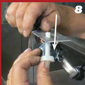
8 Remove Plunger Assembly and Stem from Valve Body.
